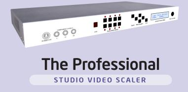
This professional video scaler/video format converter can receive and select between 8 different video sources. Multiple zoom, aspect ratio, brightness/contrast/colour saturation, gamma correction, and picture enhancement settings can be adjusted for each video source. The Scaler will output the source video to a digital (HDMI/DVI) and to an analog HD Component or VGA device.
